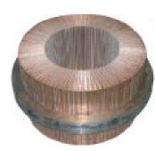
Copper and mica segment pack is then compressed under significant tonnage using a bull ring, machined to the smallest calculated diameter. This ensures maximum stability in operation.
